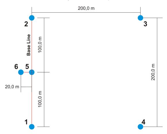
Note: It is essential for accurate speed measurement that all pylons be absolutely vertical in order to prevent course length differences with altitude.
