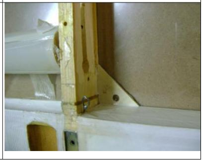
ON THE CENTRAL RIB, TO FILL WITH SOME BALSA WOOD THE EMPTY SPACES
