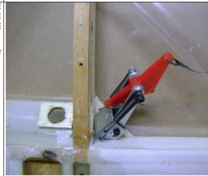
FIX THE SHUT BY THE BOLTS ON THE CENTRAL RIB AND REFIT THE LEDDER TANK AT THE ORIGINAL POSITION
