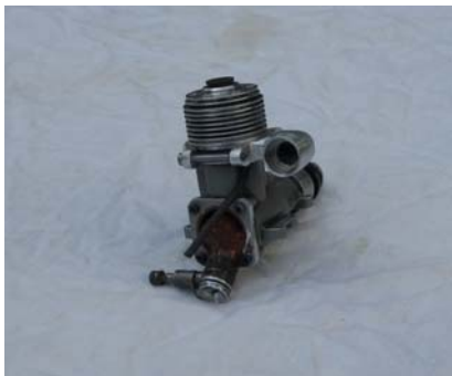
Manifold to Profi TR engine, effective length 23 mm, exhaust section area 60 mm 2 constant.
