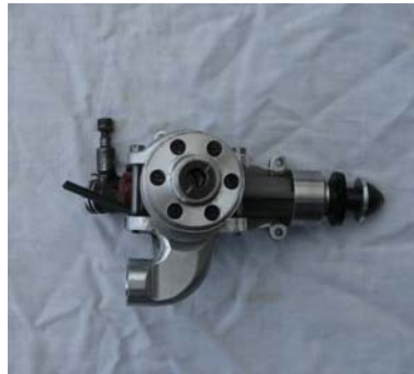
Manifold to Profi TR engine, effective length 23 mm, exhaust section area 60 mm 2 constant.
