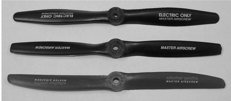
Figure 9. Master Airscrew Electric, G/F, and Scimitar propellers.
